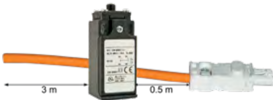
Power cable 2 x AWG 18, halogen free with door switch and Wieland female connector. Door switch: normally closed (NC), strain release, mounting plate.
